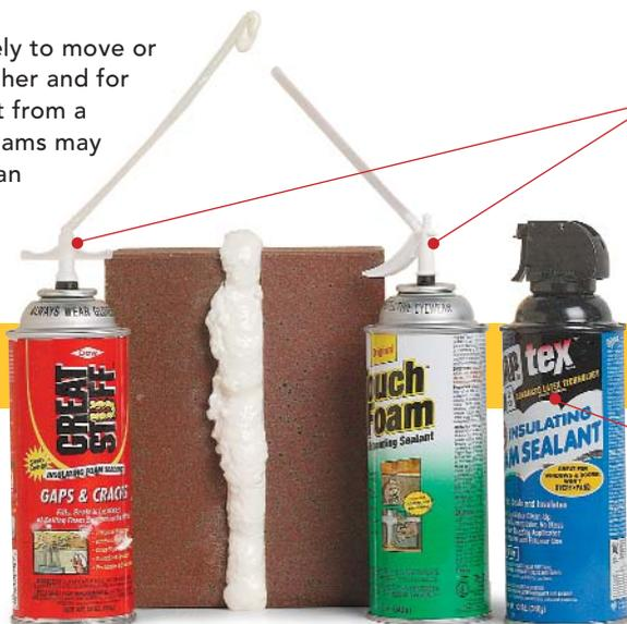
**Polyurethane spray foams** cure rigid and have an R-value up to 4.5 per in. But polyurethane foams are tricky to use because they expand as they cure. Polyurethane foams come in low, moderate, and highly expanding formulas, but even minimally expanding polyurethanes grow up to 300% before they cure.
